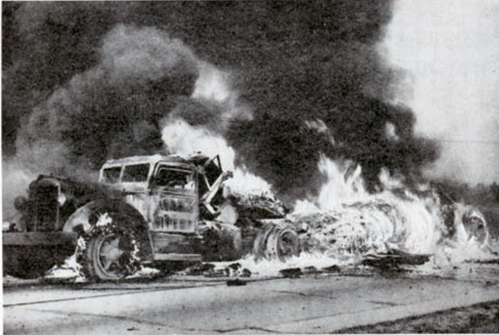
FIRE STARTED IN THIS truck's motor. A hand extinguisher couldn't prevent its spread to the cargo of fresh creamery butter. Loss to the truck and cargo was estimated at $35,000.
